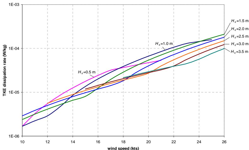
the TKE dissipation rate is high enough to cause early transition of the flow along the keel.
