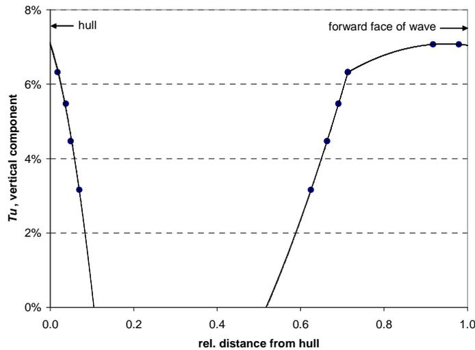
**Figure 3. Turbulence level in the bow wave on a horizontal line  $0.03 \cdot B$  below the crest at 7% of ship length behind the bow**
