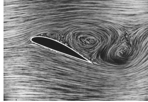
Figure 1. separated flow behind a wing section Photo: DLR, 1915, CC-BY 3.0
